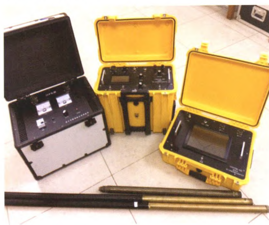
图 1 三分量 TEM 整流器、发射机、接收机及探头 Fig.1 Rectifier, transmitter, receiver and probes of the thre-component TEM system
