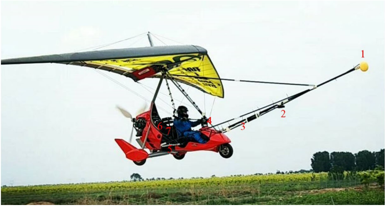
1—铯光泵磁探头;2—磁通门三分量传感器;3—实时差分 GPS;4—导航显示屏;5—高度计;6—数据采集器;7—磁补偿器 1—cesium optical pump magnetic probe;2—fluxgate three component sensor;3—real-time differential GPS antenna;4—navigation display;5—altimeter;6—data collector;7—compensator
