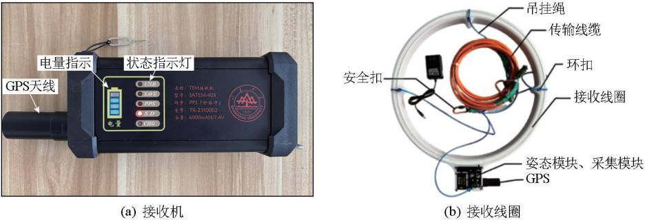
图 2 接收机与接收线圈 Fig.2 The receiver and the receiving coil
