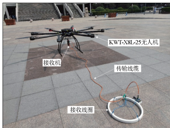
图 4 半航空瞬变电磁接收系统集成于无人机平台 Fig.4 Semi-airborne TEM receiving system integrated with UAV
