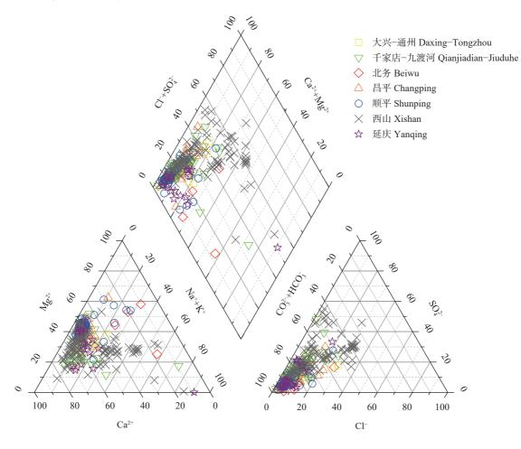
图 2 研究区水样水化学 Piper 图 Fig.2 Piper plot of groundwater in different karst water systems of the study area
