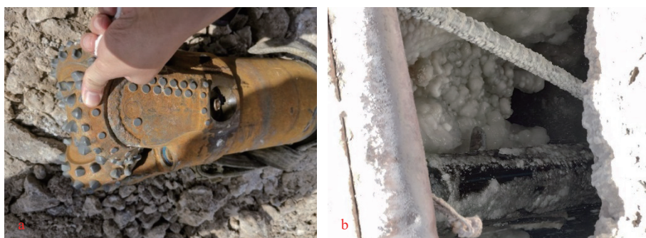
图 7 钻具腐蚀(a)及井壁结垢(b) Fig.7 Corrosion of drilling tools (a) and well wall scaling (b)
