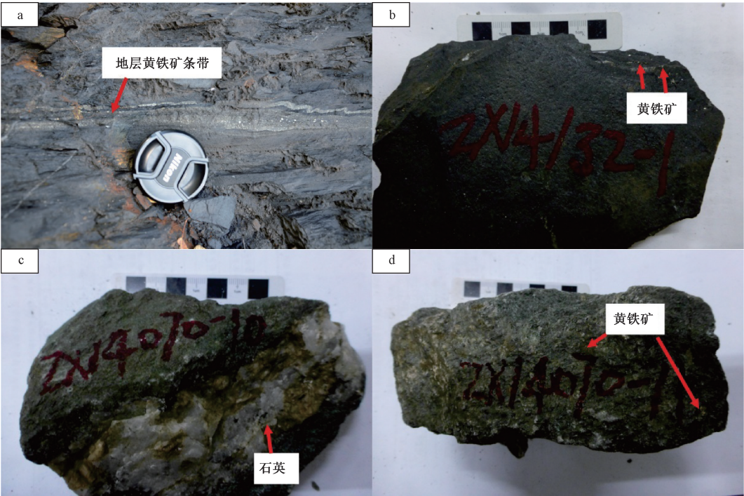
图 5 烂木沟矿区地层中黄铁矿及矿石中黄铁矿和石英 Fig. 5 Pyrite and quartz in the ores and pyrites from the strata in the Lanmugou mining area
