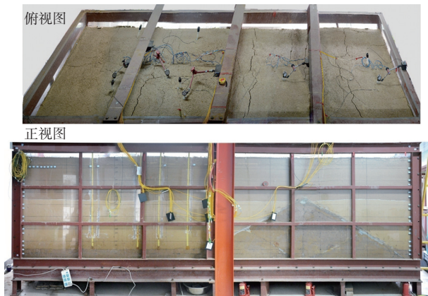
图 17 大型地裂缝物理模型系统 (俯视图与正面图) Fig. 17 Physical modeling system for large-scale earth fissures (top and front views)
