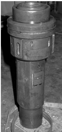
图 6 跟管钻进下套管用套管送入工具 Fig.6 Casing running tool in casing-while-drilling
