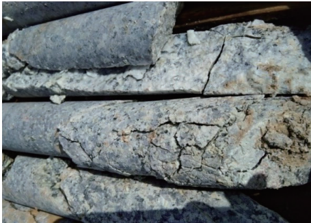
图 3 裂隙发育地层岩心 Fig.3 Cores from fracture-developed formation
