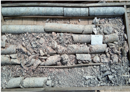
图 2 破碎地层岩心 Fig.2 Cores from broken formation
