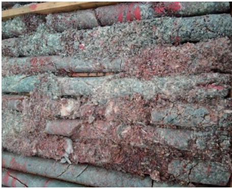
图 1 水敏性蚀变地层岩心 Fig.1 Cores from water-sensitive altered formation
