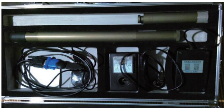
图 2 BZM 电子多点测量仪 Fig.2 BZM electronic multi-point thermometer
