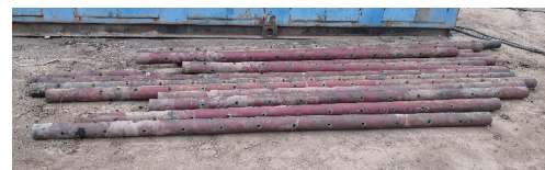
图5 射孔后的射孔枪 Fig.5 Perforating gun after use
