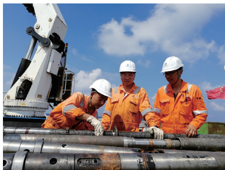
图4 回转式球阀保温保压取样钻具现场调试 Fig. 4 On-site commissioning of the rotary ball valve pressure-temperature core sampler
