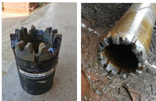
图3 金刚石齿轮钻头试验应用前后(已处理) Fig.3 Diamond gear bits before and after test application (treated)
