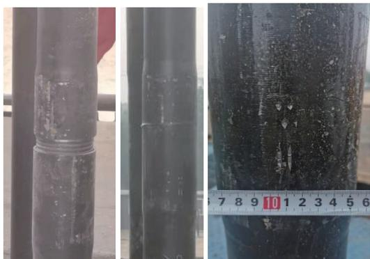
图2  $\text{O}114\text{ mm}$  绳索取心钻杆对扣、上扣情况Fig.2 Twining and screw on condition of  $\text{O}114\text{ mm}$  wire-line coring drill pipe
