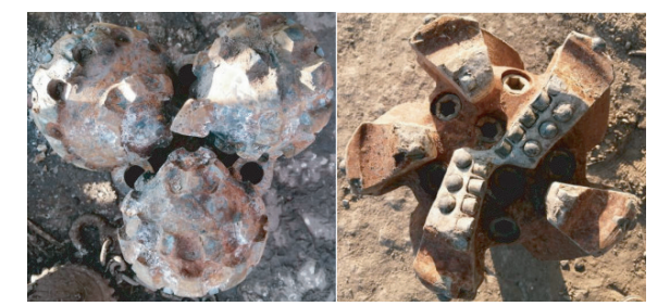
图 1 遇砾石磨损严重的钢齿牙轮和常规 PDC 钻头 Fig.1 Severely wore teal tooth and conventional PDC bit when encountering gravel
