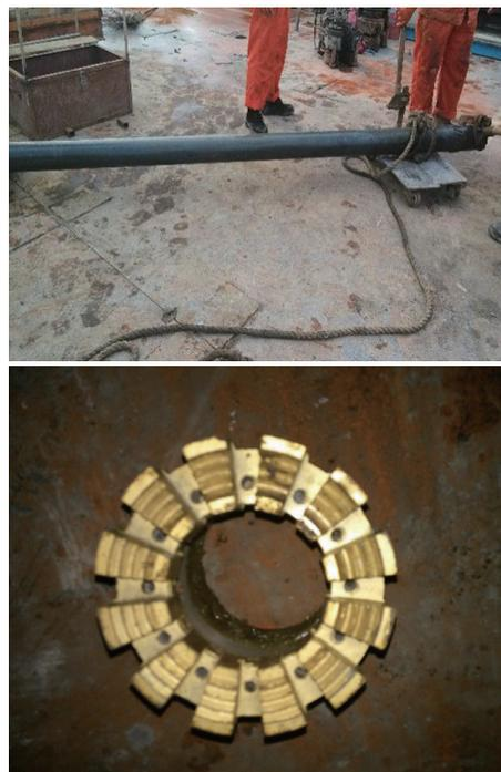
图6 CSDP-02井S-P绳索取心钻具和钻头
