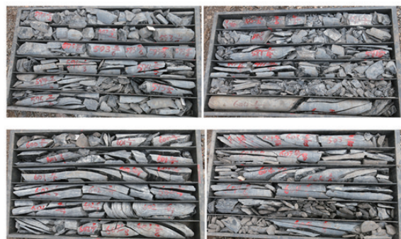
图3 孔深 1770~1820 m 垂直节理裂隙发育地层岩心 Fig.3 Cores from vertical joint and fracture developed formation at depth of 1770m to 1820m
