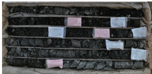
图 3 1270~1276 m 孔段取出的炭质泥岩及煤层岩心 Fig.3 Carbonaceous mudstone and coal seam core from the 1270~1276m hole section
