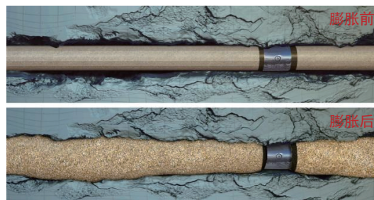
图1 GeoFORM防砂系统原理(来源于贝克休斯公司官网) Fig.1 Schematic diagram of GeoFORM sand control system (from the official website of Baker Hughes)
