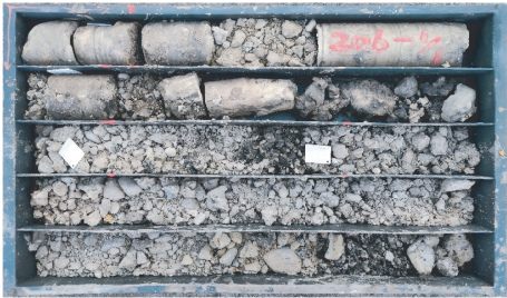
图 5 极松散含砾砂层岩心 Fig.5 Core of extremely loose gravel sand layer
