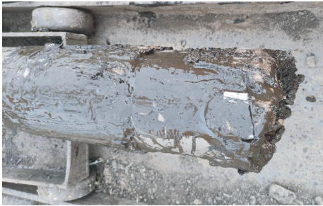
图6 严重泥包的钻头及钻具 Fig.6 Drill bits and drilling tools with severe mud inclusion
