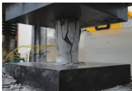
图6 注浆固结体圆柱试样的破坏特征 Fig.6 Failure characteristics of cylindrical specimens of grouting consolidated body
