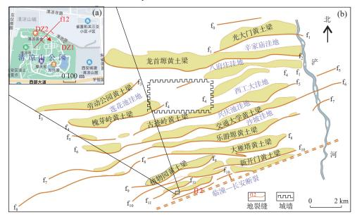
图 1 清凉山 f12 地裂缝钻孔位置图(a)和西安地区地裂缝分布示意图(b)(据王璐, 2010) Fig. 1 (a) Drilling locations of f12 fissure and (b) Distribution of ground fissures in Xi'an area
