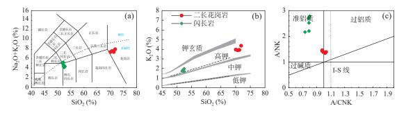
图5 乌孙山地区花岗岩和闪长岩 TAS 图解(a), K<sub>2</sub>O-SiO<sub>2</sub>(b)和 A/NK-A/CNK(c)图解(引自 Bao et al., 2018) Fig. 5 (a) The TAS, (b) K<sub>2</sub>O-SiO<sub>2</sub> and (c) A/NK-A/CNK diagram of granite and diorite in Wusunshan area
