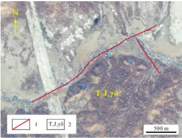
图 2 河道突变 GF-1 遥感影像图 Fig. 2 GF-1 remote sensing image of river channel change 1—断层(fault); 2—晚三叠世-早侏罗世花岗闪长岩(Late Triassic-Early Jurassic granodiorite); 波段组合(band combination): R (4) G (3) B (2)
