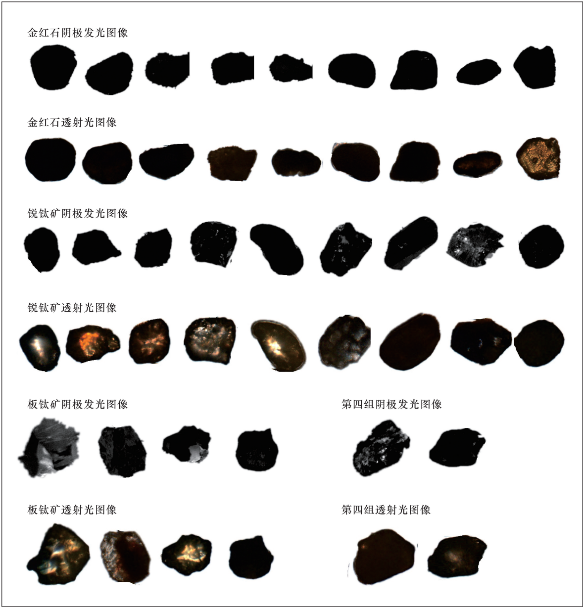
图 4 桂中铝土矿 TiO 2 同质异象矿物透射光及阴极发光图像 Fig. 4 Transmitted light and cathodoluminescence photos of the TiO 2 polymorphs from the bauxite deposit in central Guangxi
