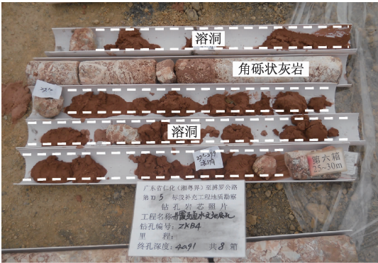
图 5 钻孔揭示溶洞 Fig. 5 Boreholes revealing the development situation of karst cave
