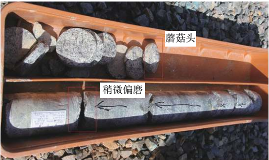
图 3 岩心偏磨和蘑菇头 Fig. 3 Core bias grinding and mushroom head
