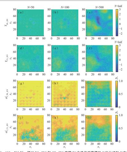
图 3 当 N=50, 100, 500 时,通过 DL\_iES 和 CL\_iES 在第 20 次迭代后获得的 Y 估计场和 Y 方差  $(\sigma_Y^2)$  估计场 Fig. 3 Maps of Y fields and Y variance  $(\sigma_Y^2)$  estimated through DL\_iES and CL\_iES at the 20th iteration when N=50, 100, 500
