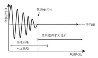
图 3 不同尺度地层介质特性变化示意图 (据文献 [7] 修改 ) Fig. 3 Schematic diagram of changes in the characteristics of geological media at different scales (modified after Ref. [7])
