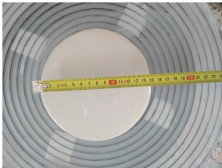
图 2 流动度、可泵期测试 Fig. 2 Flowability and pumpability tests
