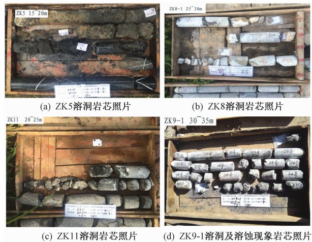
图 5 杨村子研究区钻孔岩芯照片 Fig.5 Borehole core photos of boreholes in Yangcun study area
