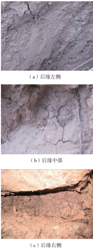
图 4 凉水井滑坡滑面形态特征 Fig. 4 Morphological characteristics of the sliding surface of the Liangshuijing landslide
