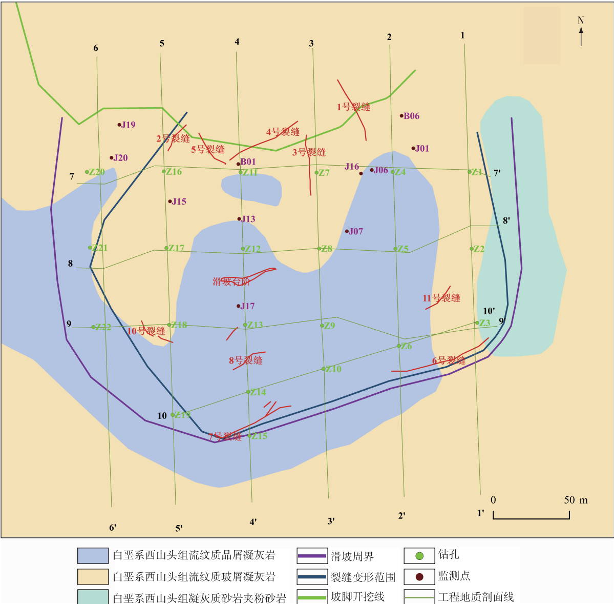
图 4 金华市某岩质滑坡监测点平面布置图 Fig. 4 Monitoring map of a rock landslide in Jinhua City
