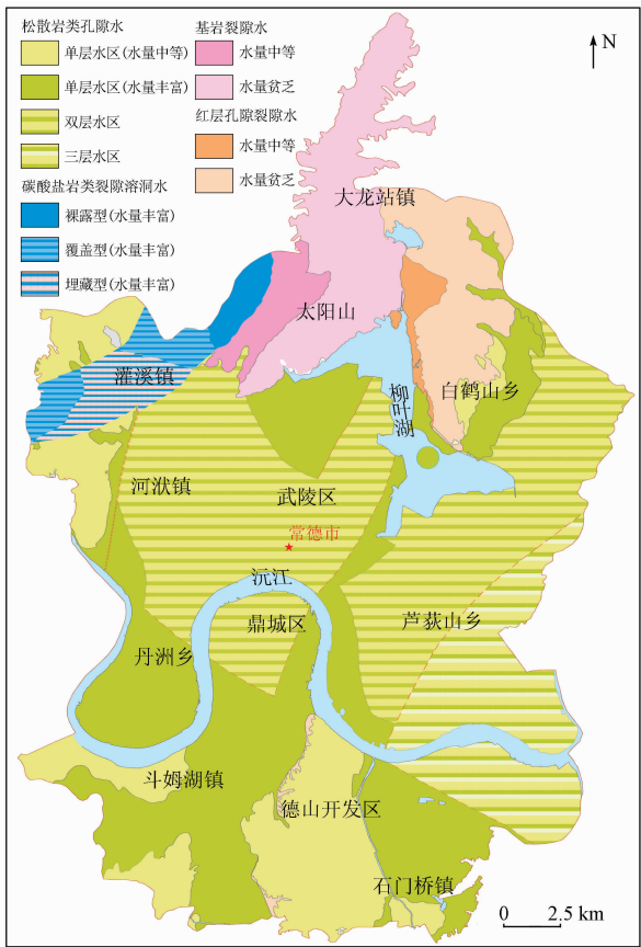
图 3 研究区地下水类型及富水性分带 Fig. 3 Zoning map of groundwater types and water abundance in the study area
