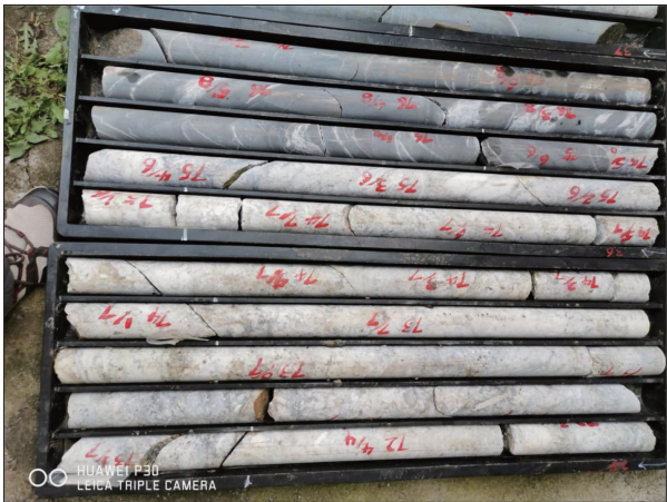
图 2 四川省马尔康马纳一带新发现的含锂辉石伟晶岩 (2023 年 9 月,白色岩心主体为含锂辉石伟晶岩) Fig. 2 Newly discovered spodumene pegmatite in Mana of Maerkang in Sichuan Province (September, 2023, the white core is mainly composed of spodumene pegmatite)
