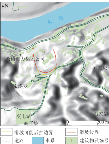
图 5 老电厂滑坡建筑物分布 Fig.5 Buildings distribution of Laodianchang landslide
