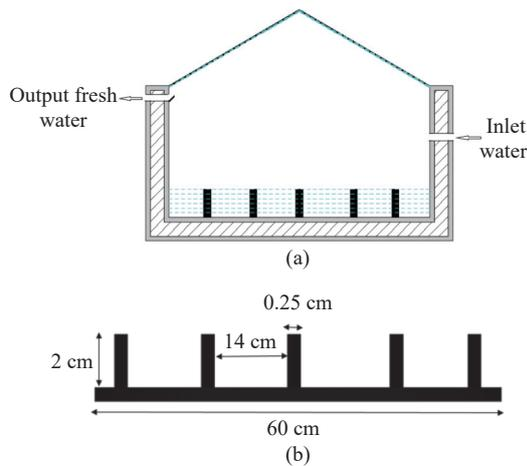
**Fig. 2** (a) Schematic diagram of the pyramid solar still with fins in the basin; (b) Detailed dimension of the fins
