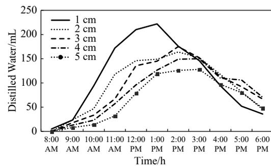
Fig. 6 Variation of hourly freshwater productivity for pyramid solar still with different water depths
