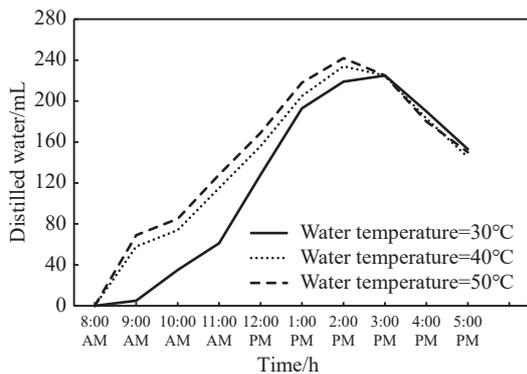
Fig. 8 The effect of changing inlet water temperature from 30°C to 50°C on solar still productivity
