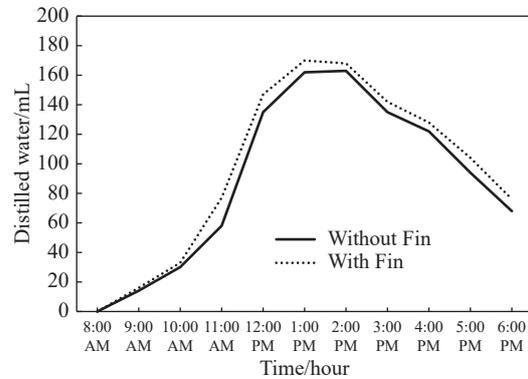
Fig. 9 Effect of fins on productivity in the pyramid solar still
