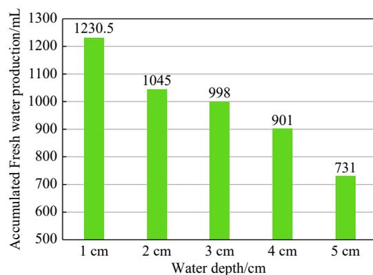
Fig. 7 Total amount of fresh water produced by the pyramid solar still with different water depths
