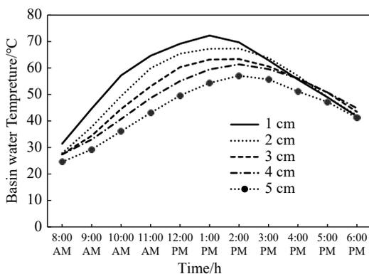
Fig. 5 Variation of basin water temperature during experimental hours for different water depths
