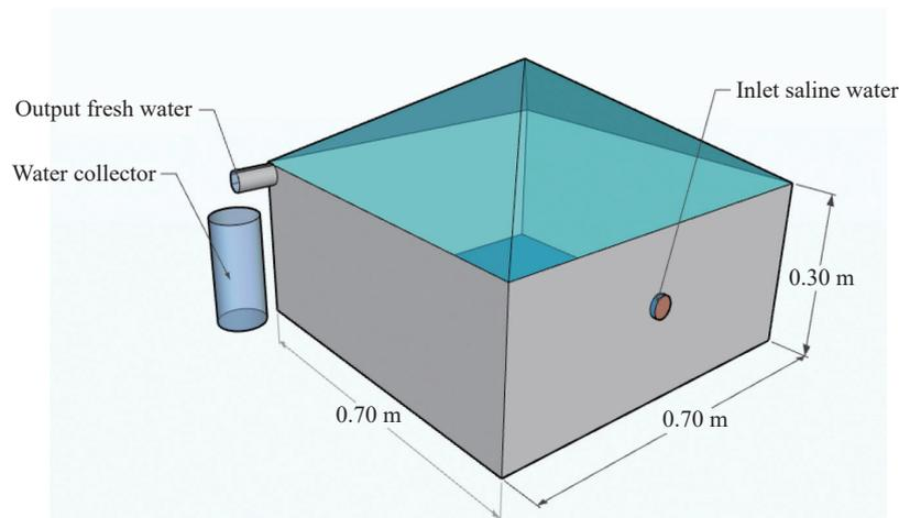
Fig. 1 Pyramid solar still used in the experiment
