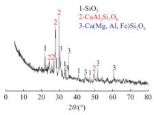
图 8 较佳条件下样品的 XRD Fig.8 XRD of samples atoptimal condition
