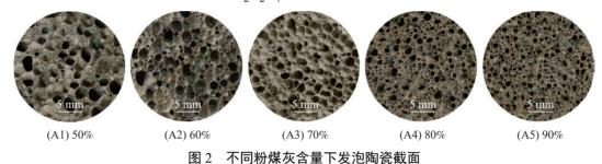
Fig.2 Cross-sections of foamed ceramics with different fly ash content
