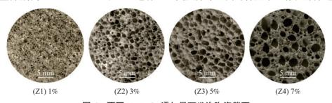
图 6 不同  $Na_2B_2O_7$  添加量下发泡陶瓷截面 Fig.6 Cross-sections of foamed ceramics with different  $Na_2B_2O_7$  addition
