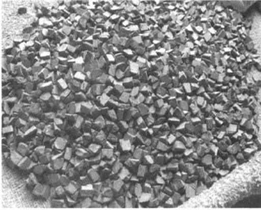
图1 低品质刚玉 Fig. 1 Low-quality corundum
