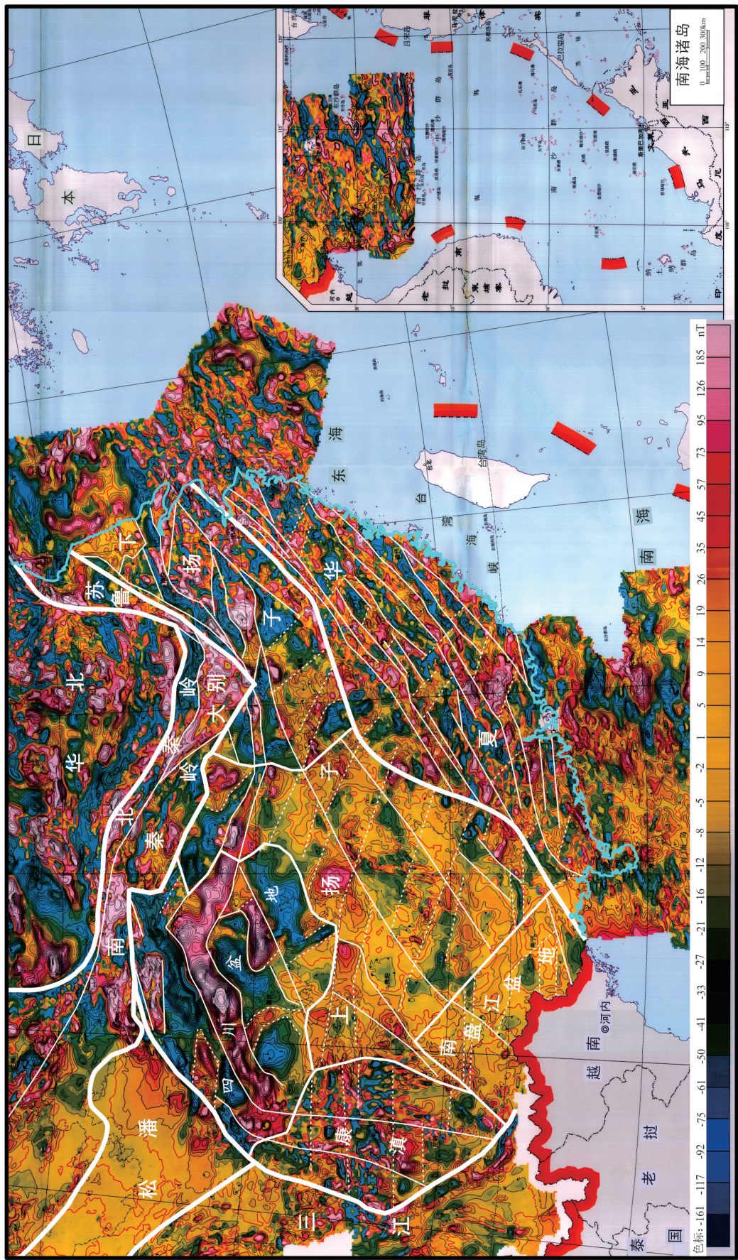
图 4 华南及邻区航磁图(中国国土资源航空物探遥感中心, 2004)与构造解译 Fig. 4 The aeromagnetic map and its structure interpretation of South China and adjacent areas
