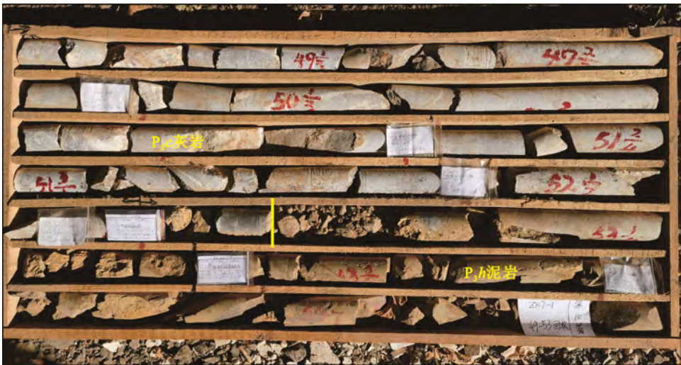
图 2 小天井锰矿 ZK7-1 灰岩与泥岩接触带 Fig. 2 ZK7-1 zone of contact between limestone and mudstone in the Xiaotianjing Mn deposit
