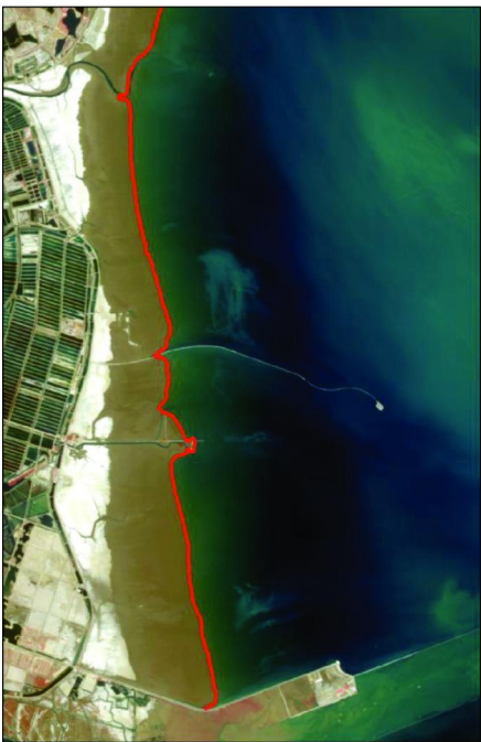
图 3 基于 Canny 边缘检测的水边线提取结果 Fig. 3 Waterline extraction result based on Canny edge detection
