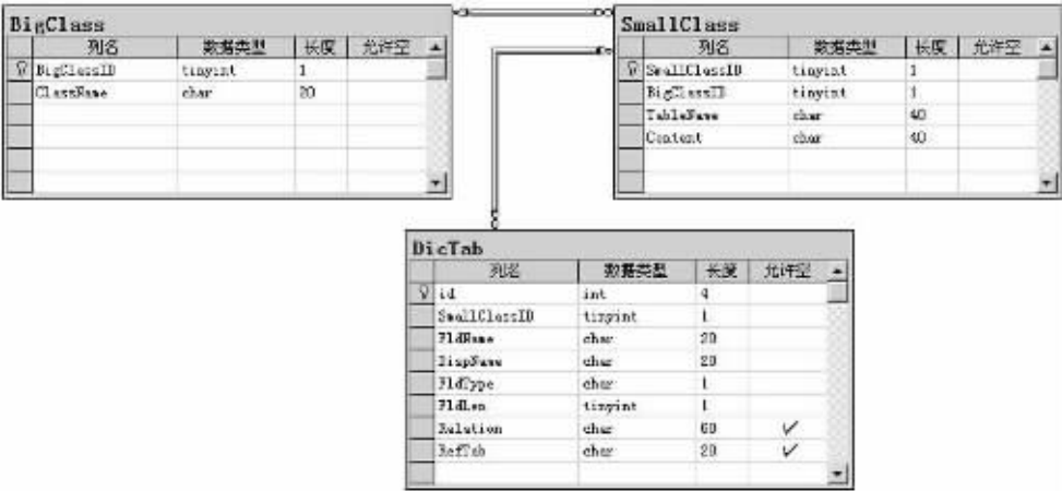
图1 BigClass,SmallClass 与 DicTab字典表之间的关系 Fig.1 Relations between BigClass table, SmallClass table and DicTab dictionary table
