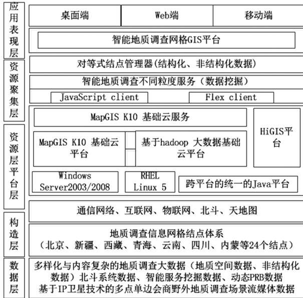
图2 基于大数据技术的智能地质调查云(网格)平台架构 Fig. 2 Cloud (grid) platform architecture of intelligent geological survey based on big data tech
