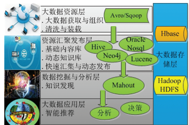
图3 基于大数据技术智能地质调查数据发现与服务总体框架 Fig. 3 Overall framework of intelligent geological survey for data discovery and services based on big data tech
