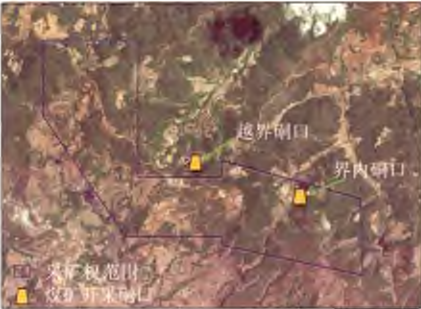
图 5 采矿权界内与越界的煤矿开采硐口影像特征 Fig.5 Imaging features of cave mouth innor and cross the border of mining right
