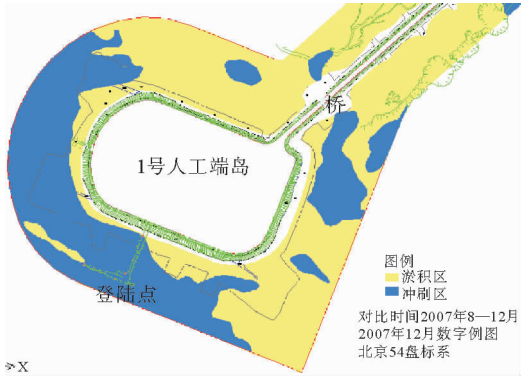
图 9 1 号人工端岛区海底变化图(2007 年 3—12 月) Fig. 9 Seabed topographic variation of the artificial island (from March to December, 2007)
