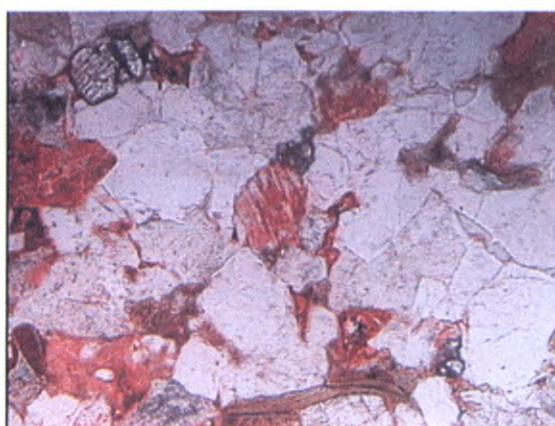
评158井670.77m, 溶蚀粒内孔隙
