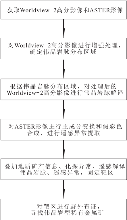
图 3 伟晶岩型锂矿遥感找矿方法技术流程图 Fig. 3 Technical process of remote-sensing prospecting for pegmatite type Lithium deposit
