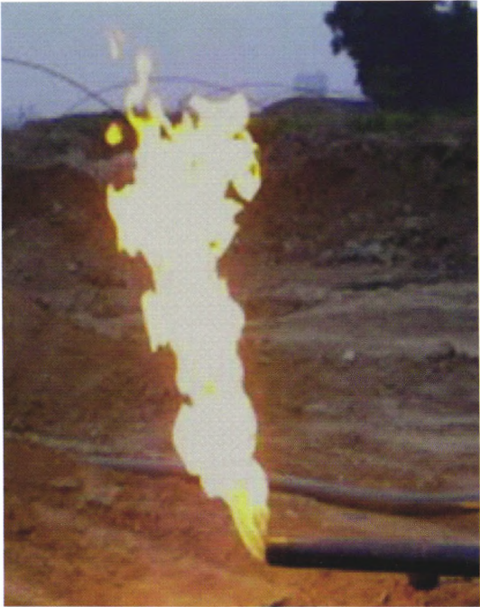
图 4 地热水伴生生物甲烷气点火照片 Fig. 4 Photos for the ignition of biogenic methane gas accompanying geothermal water
