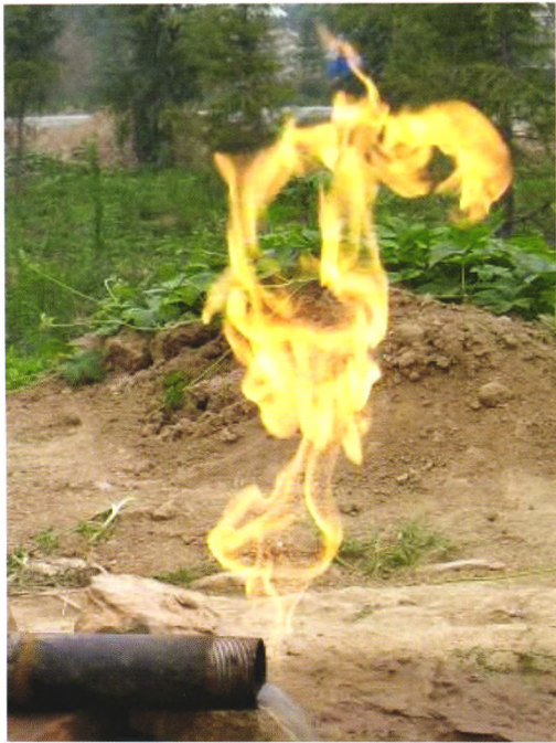
图 4 地热水伴生生物甲烷气点火照片 Fig. 4 Photos for the ignition of biogenic methane gas accompanying geothermal water
