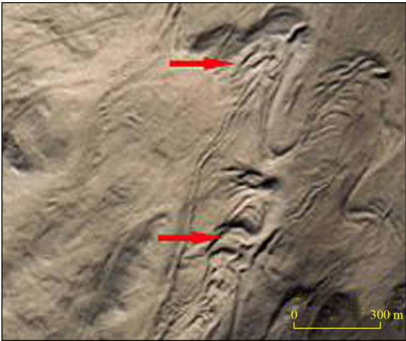
图 10 融冻作用形成的舌状泥流影像 (GF-1 遥感图像) Fig. 10 Image of ligulate solifluction created by thaw - freeze action
